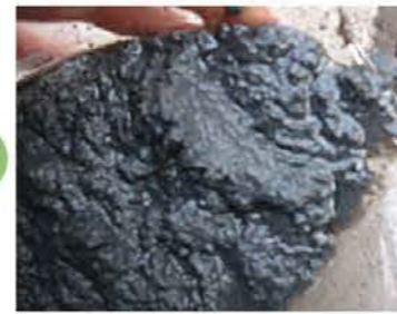
濃縮後 Sludge Thickening
